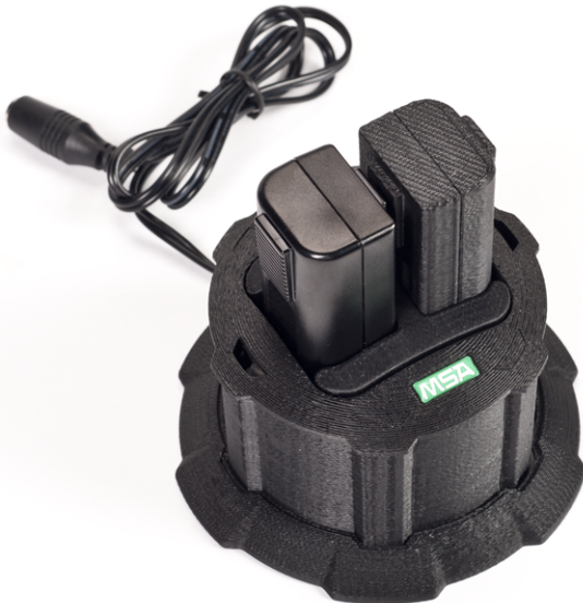
Fig. 12 Battery insert placement in the Charger nest
